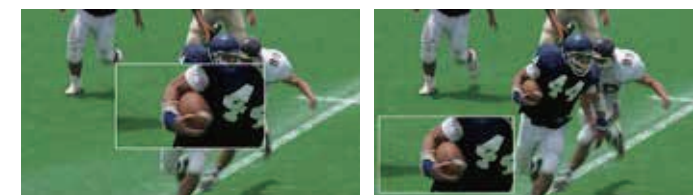
Pixel-to-Pixel display on the VF screen. The display position is selected from the center area and four quadrant area.
