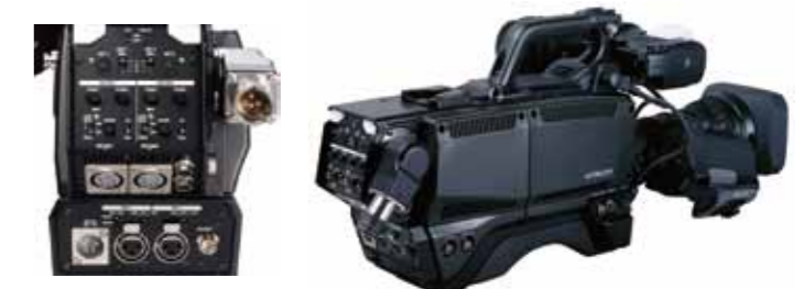
The SK-HD1000 incorporates heavy duty mounts for both the ENG and Studio viewfinders.
